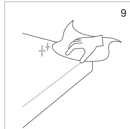
**EN:** Clean the surface of the shower tray very well. Scrape the gel-coat on the defect area off with scraper. Use the sandpaper to wrap the foamed block around, then sand the defect area. Clean the surface with a dry lint-free cloth, then apply for acetone or ethyl alcohol in water with the lint-free cloth. Surface must be totally clean and dry.
